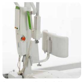
The emergency stop can be easily reached, but its position on the side reduces the risk of it being pressed accidentally. The electrical emergency lowering control is also easily reached.
